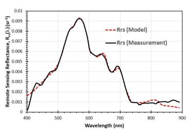
Figure 2: Measured reflectance spectrum (black solid line) and best-fit computed reflectance (red dashed line) using the Gaussian peaks model for phytoplankton absorption.
