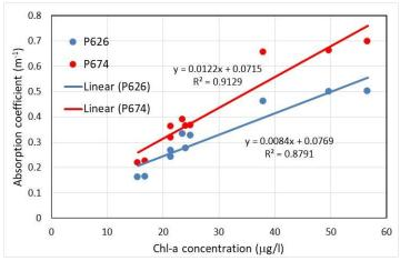
Figure 3: Regressions of the Gaussian peak strengths at 674 nm and 626 nm with chlorophylla concentration.
