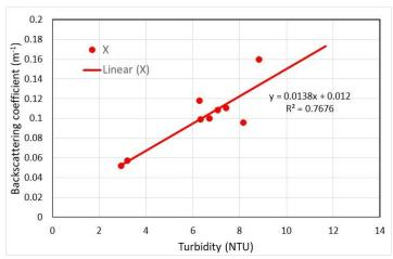
Figure 4: Regression of particulate backscattering coefficient with water turbidity.
