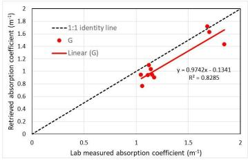
Figure 5: Regression of CDOM absorption coefficient retrieved from reflectance with Labmeasured CDOM absorption.
