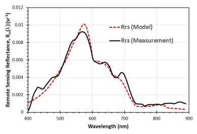
Figure 1: Measured reflectance spectrum (black solid line) and best-fit computed reflectance (red dashed line) using the conventional model for phytoplankton absorption.
